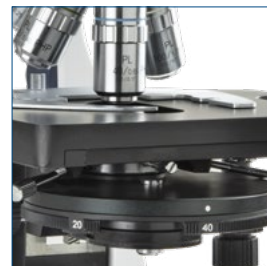
Zernike phase contrast condenser with filter holder
